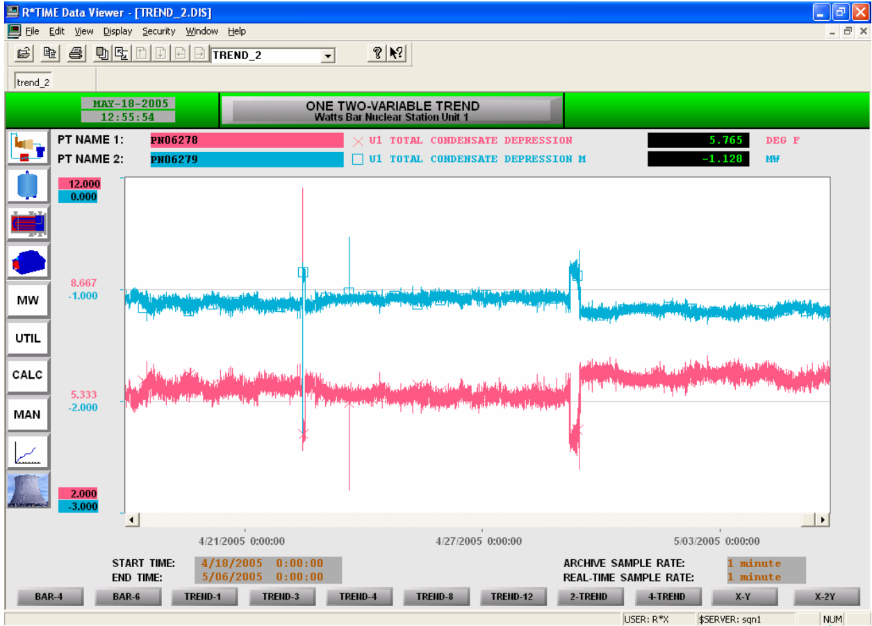
Figure 5 –Watts Bar Condensate Depression Trends
