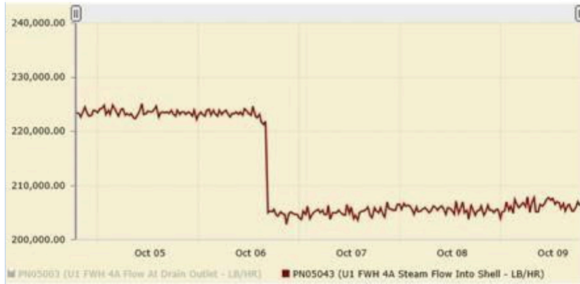
The FAMOS graph showing Exelon's drop in power generation due to bellows rupture.
