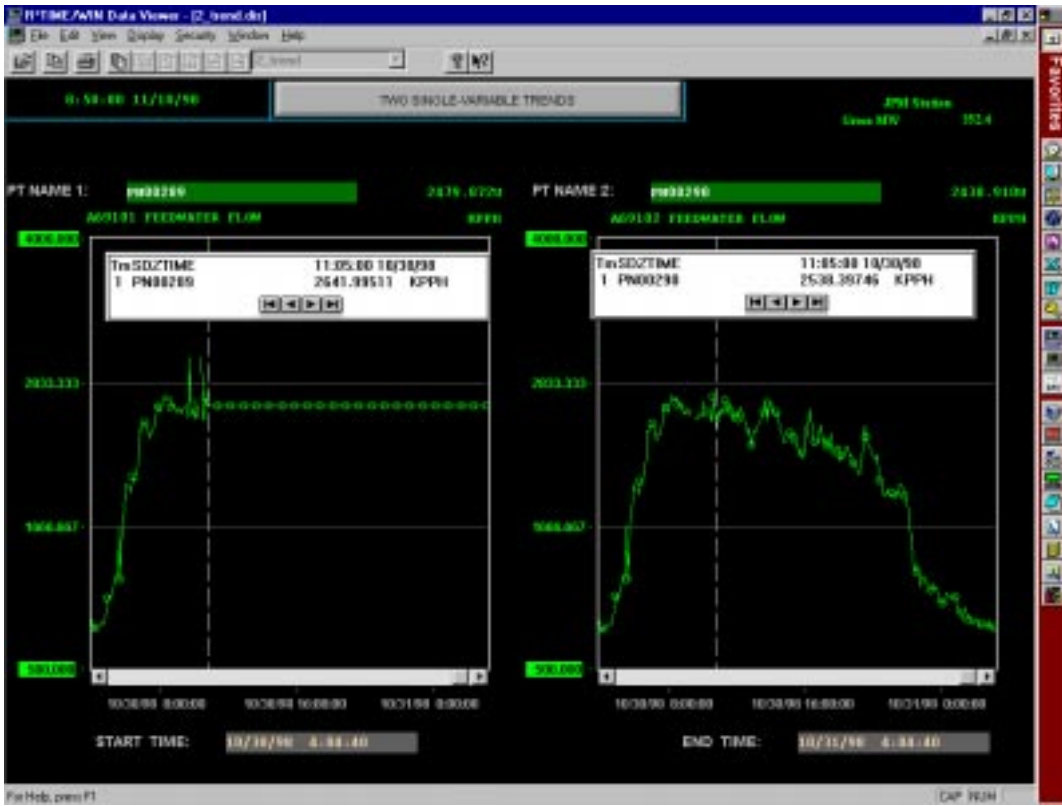
Figure 7 PMAX Trend of Two Feedwater Transmitters
