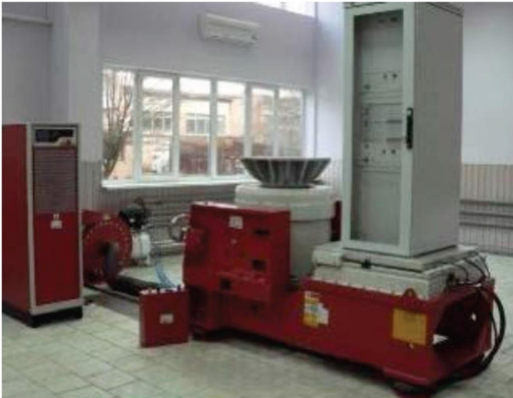
Electrodynamic Vibration Table V875-440 HBT Combo, LVD
