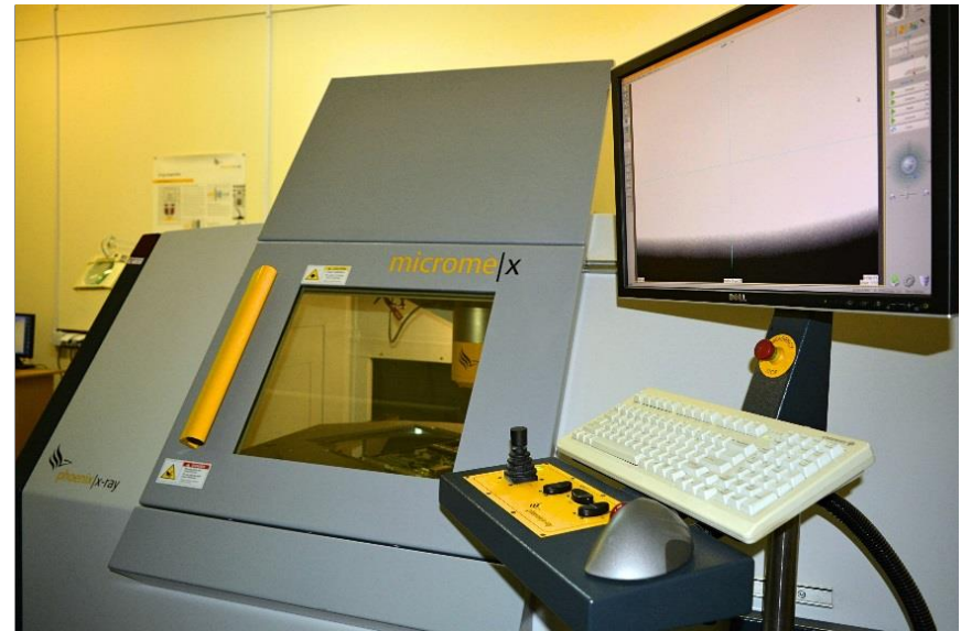
X-ray inspection system for real time inspection of solder joints
