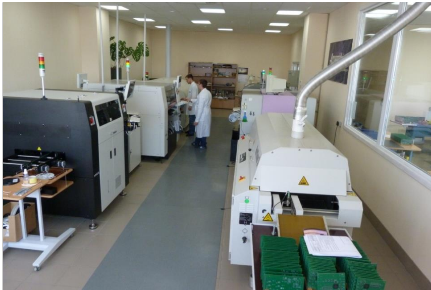
Automated production line for PCB surface mounting
