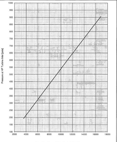
Mass Flow Rate at HP Turbine Inlet [k.lb/h]
