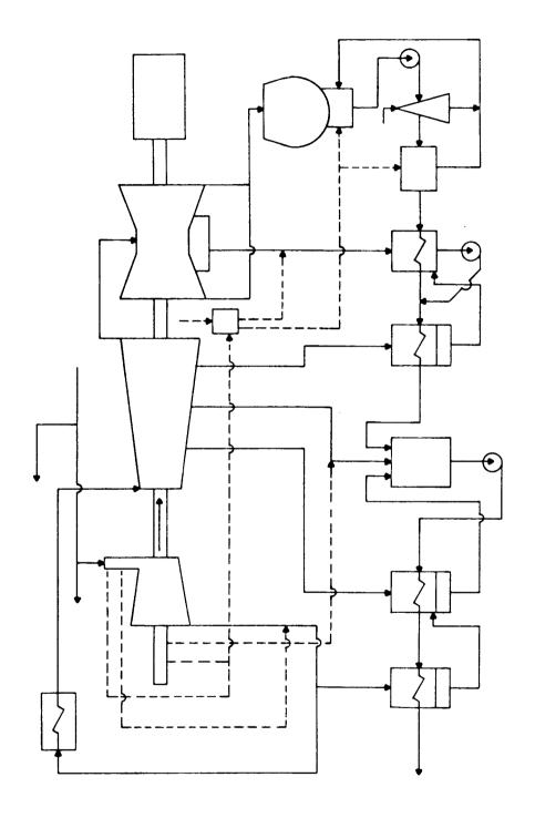
Figure 1 - Paint Creek Unit 4 Turbine Cycle Schematic
