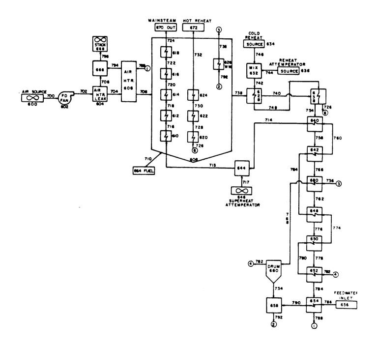
Figure 3B - Paint Creek Unit 4 PEPSE Boiler Model
