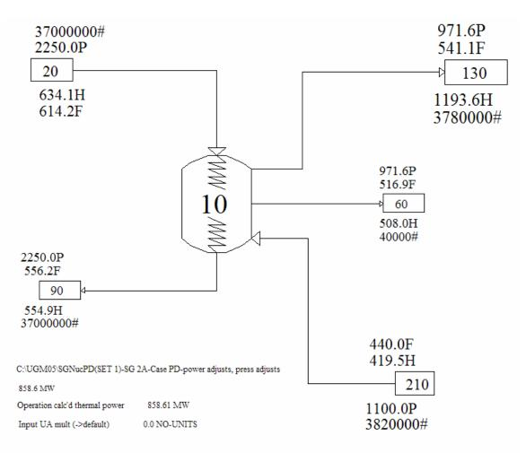
Comparison of the results of the TA and TB cases shows that the UA multiplier and the shell-side pressure are quite sensitive to the specified value of thermal power. This demonstration suggests the importance of caution in validating and verifying results of models.
