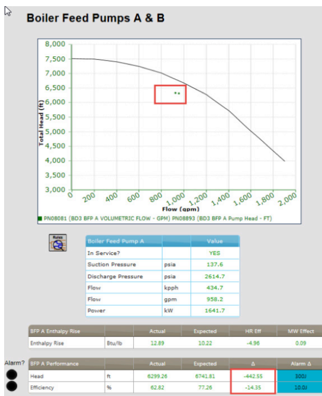
PdP shows the drop in Boiler Feed Pump efficiency.
