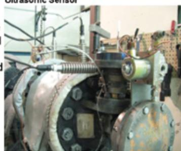
4 Ultrasonic Sensors on TR 3-stage SRV
